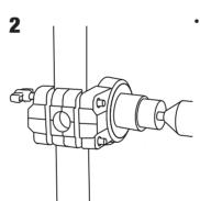
Using the 44mm arbor and holesaw, drill through the face of the door from the guide side until the drill tip exits the timber on the opposing side. Switch sides and use the exit point as the guide to continue drilling (by applying low pressure) and remove the core.
